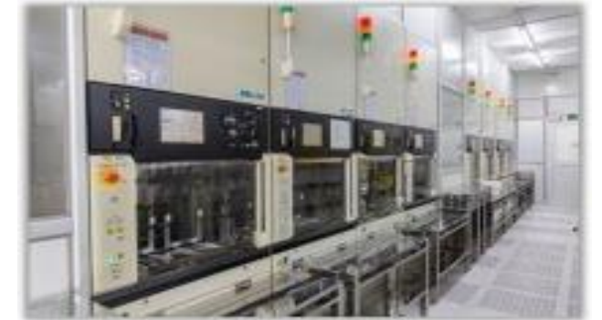
PECVD Deposition System
