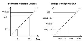
Fig. 1: Characteristics of output voltage
