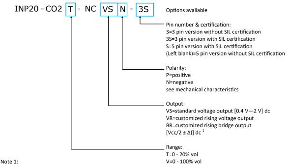
The bridge output is indicated to use when substituting a pellistor.
