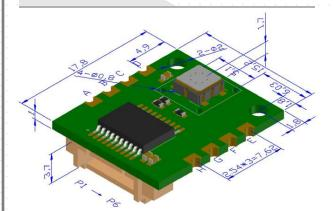
Unit: mm A: UART\_TX B: +5.0V C: NA D: SDA E: GND F: SCL G: NA H:UART-RX Pitch: 2.54mm P1: VDD P2: SCL P3:SDA P4:Rx P5:Tx P6:GND
