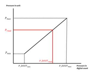
For example, the  $P_{min}$  and  $P_{max}$  for the sensor are specified as -300 and +500 clinical mmHg. The  $D_{OUT\_MIN}$  and  $D_{OUT\_MAX}$  are -26214 and +26214.
