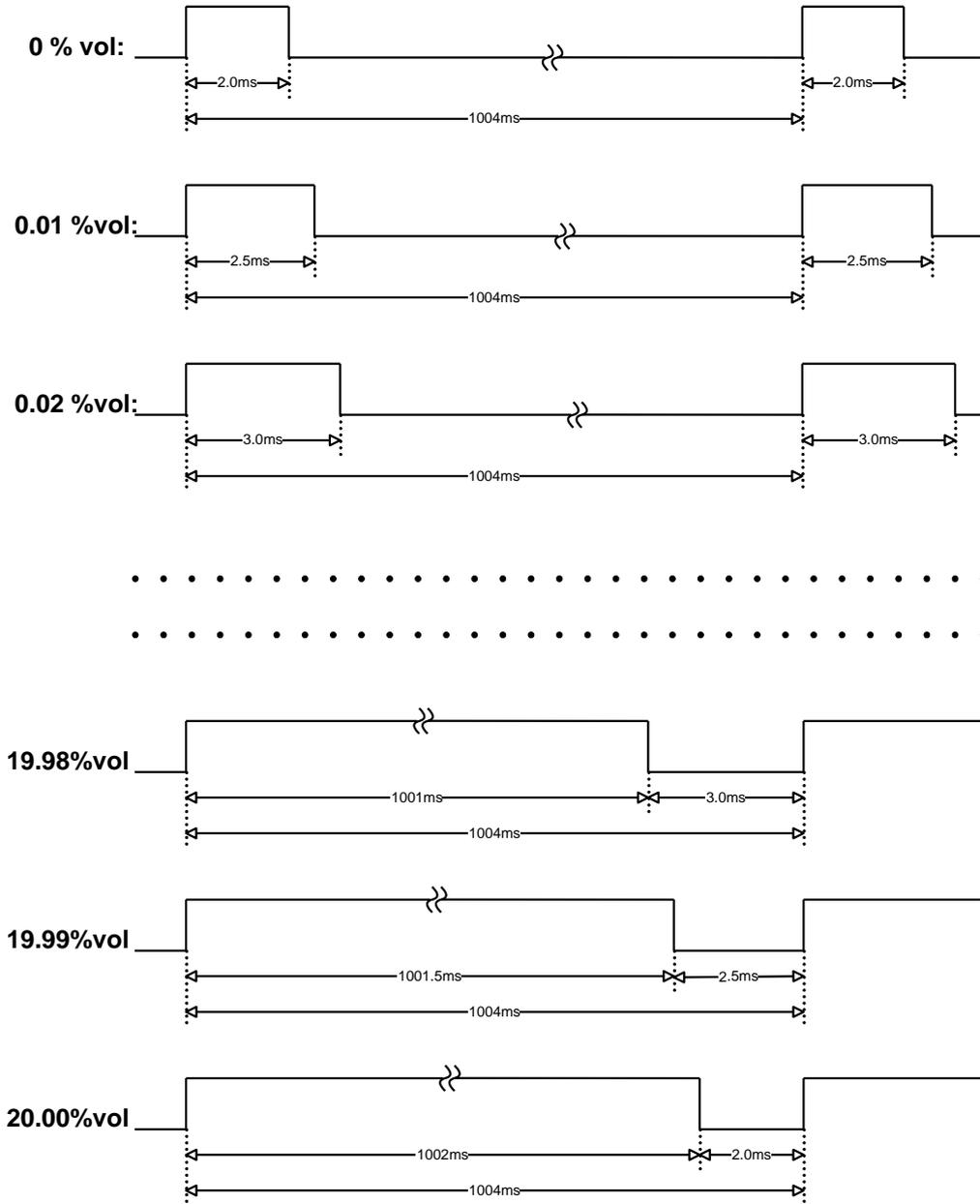
Figure 7. Senseair K33 ICB OUT1 timing diagram.
