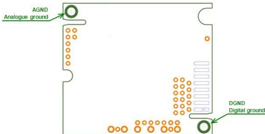
Figure 5. Senseair K33 ICB ground / shield attachment
