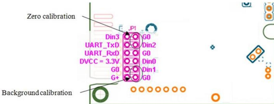
Figure 6. Senseair K33 ICB (component side) zero and background calibration inputs for calibration jumpers.
