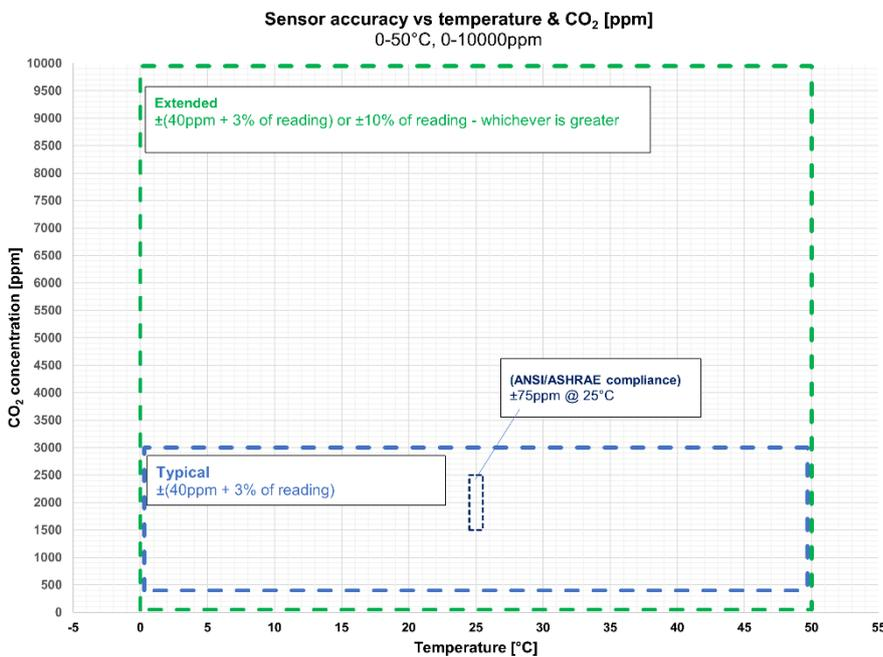
Figure 4. Accuracy over complete operating range (temperature and measurement of CO<sub>2</sub>).
