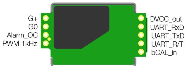
Figure 2. Pin assignment
