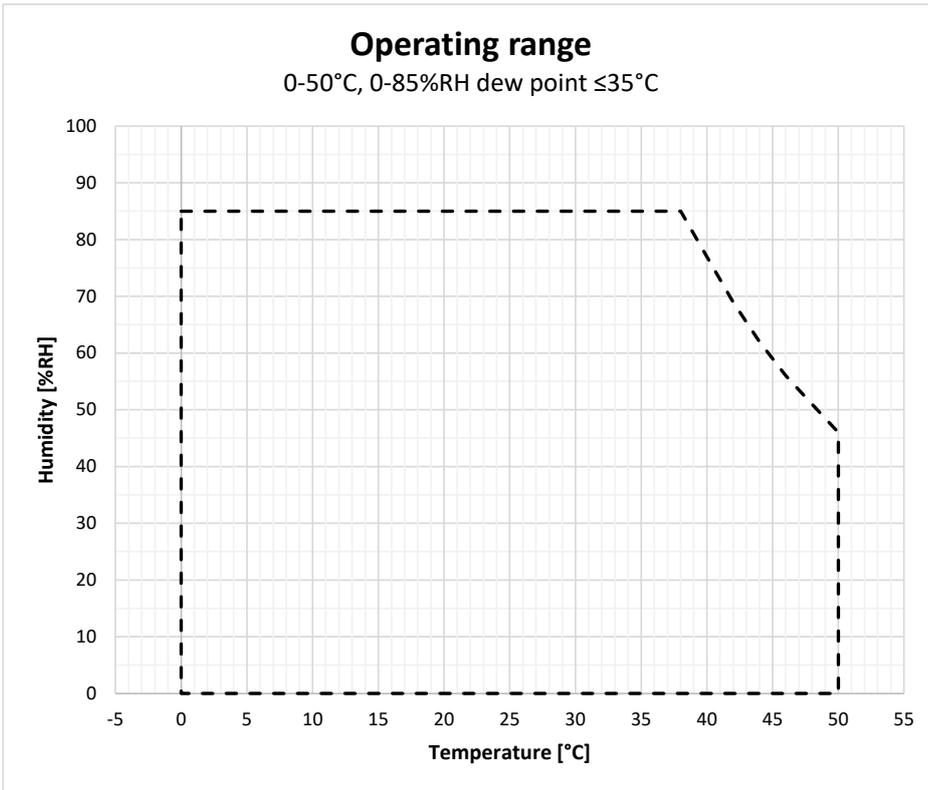
Figure 3. Operating range for specified in Table 1 accuracy.
