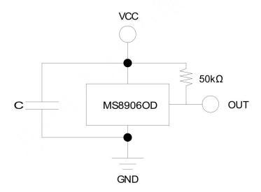
MS8906OD's pole-independent sensing technique allows for operation with either a north or south poles magnet orientation, enhancing the manufacturability of the device. The state-of-the-art technology provides the same output polarity for either pole face.
