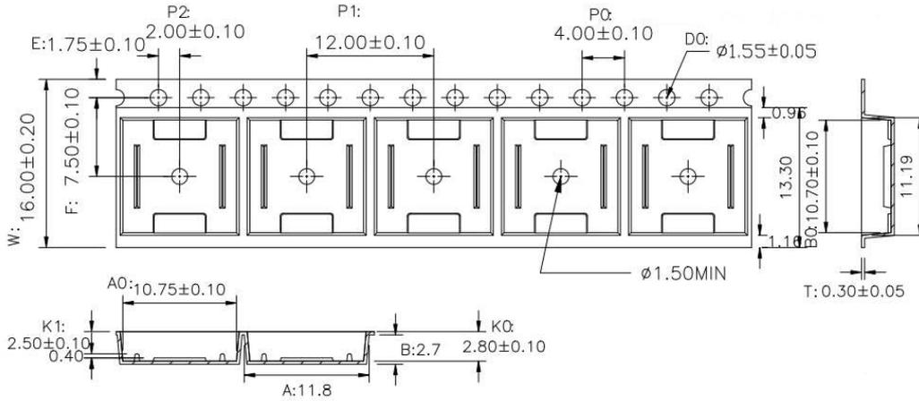
1. 10 sprocket hole pitch cumulative tolerance  $\pm 0.20$ .
