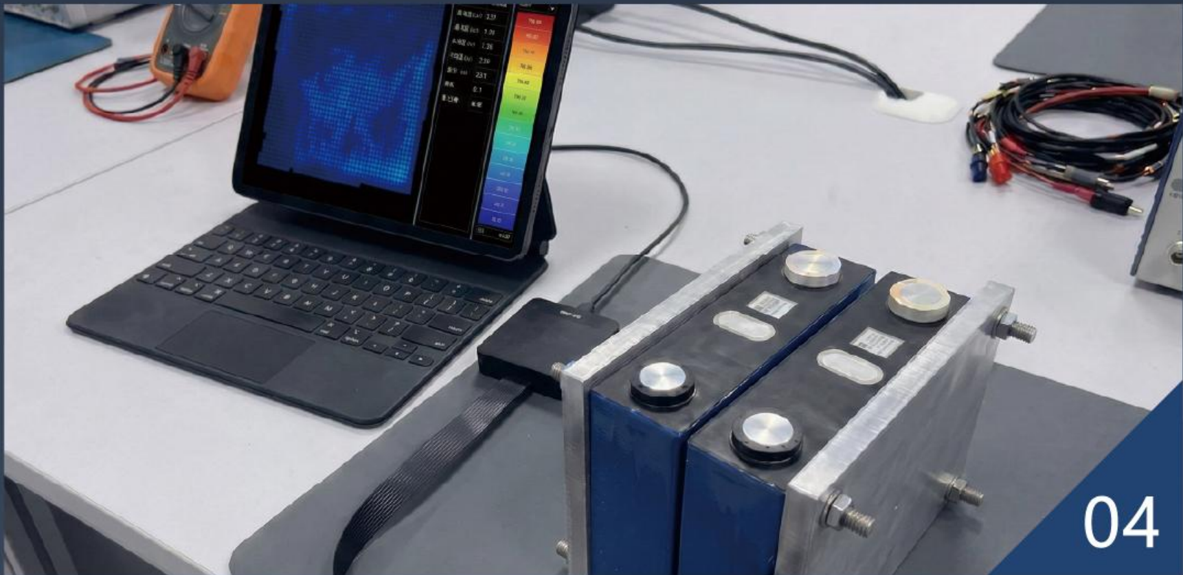
Single Cell Pressure Testing
